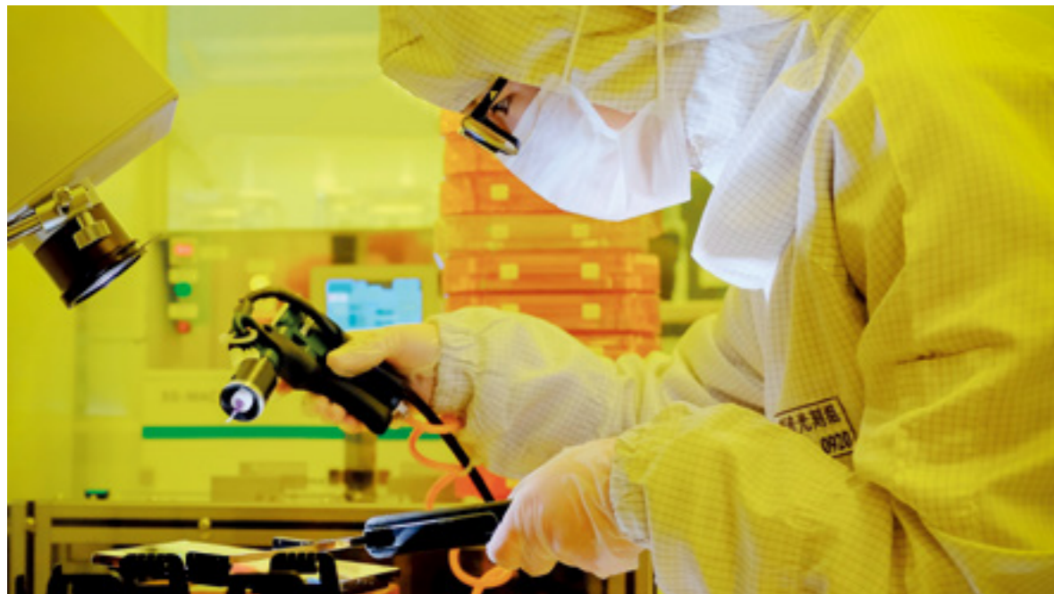
Staff of the photolithography team carefully checking the surface of the mask.
